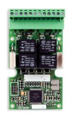
**TRD-100** Expansion card of 4 free voltage relay outputs
