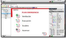
Graphics management by Vesta is an impressive change of HMI (Human Machine Interface) in fire detection panels. It makes substantially easy the events location and it allows faster actions in any case through customized virtual control dashboards.
